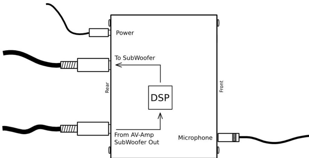
Figure 4: Setting up the ANTI-MODE 8033
