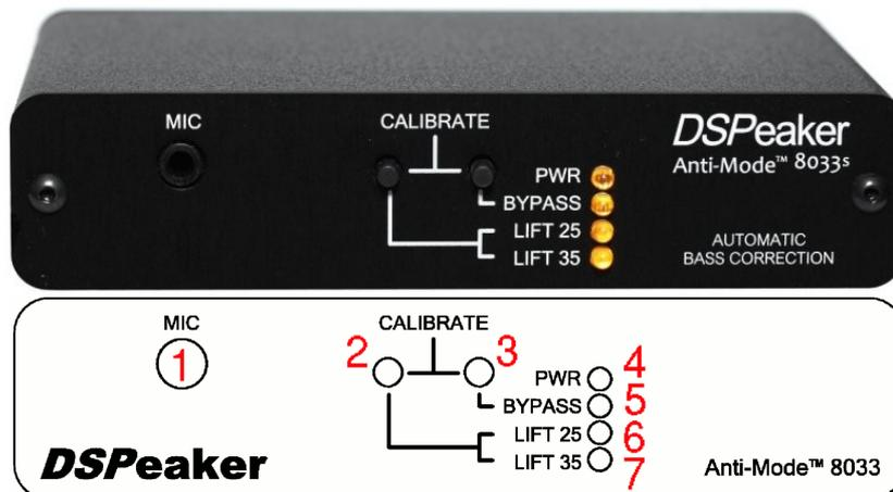
Figure 1: ANTI-MODE 8033 Front panel
