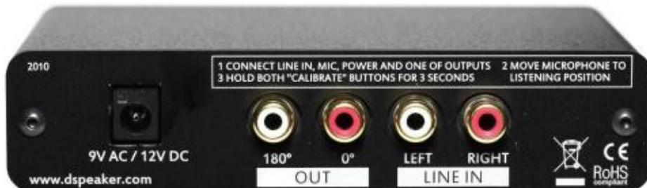
Figure 3: ANTI-MODE 8033S-II rear panel
